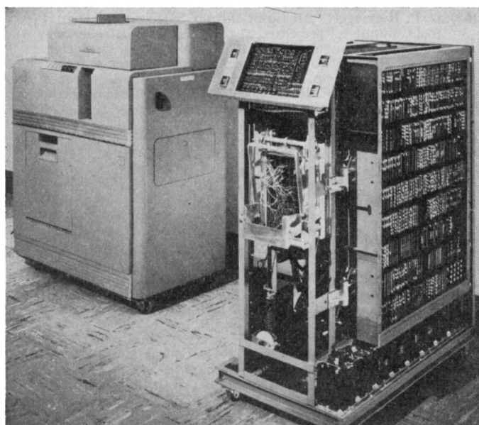
IBM's experimental all-transistor calculator. This new experimental computer is composed of a high-speed punching unit (left) and the transistorized calculating unit at right. The calculating unit is uncovered to show the bank of printed wiring panels on which the transistors are mounted. This "all-transistor" unit is approximately one-half the size of a vacuum-tube unit of comparable capacity and requires only 5 per cent as much power.
