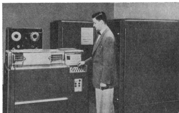
High-speed printer of the UNIVAC system for handling large volume output. It is capable of printing 600 lines per minute.
