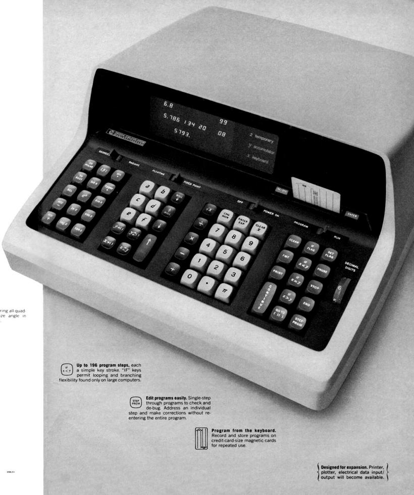
**Up to 156 program steps**, each a simple key stroke. "IF" keys permit looping and branching flexibility found only on large computers.
